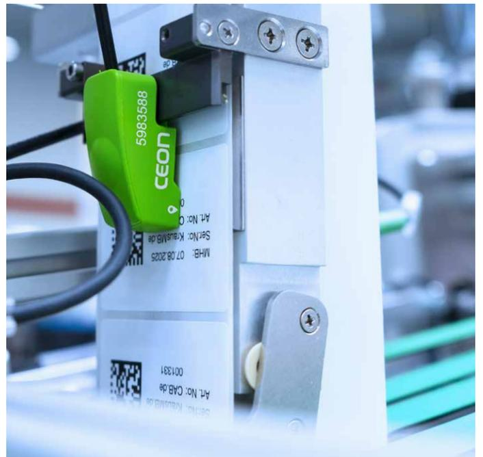
**IXOR is labeling at full speed**, whereas on its peel-off plate a sensor is detecting each label.
