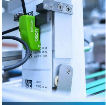
**IXOR** is labeling at full speed, whereas on its peel-off plate a sensor is detecting each label.
